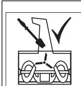
Only clean the discharge chute with cleaning utensils..
