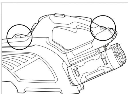
A carrying belt can be attached to the eyelets (not included in the scope of delivery).
