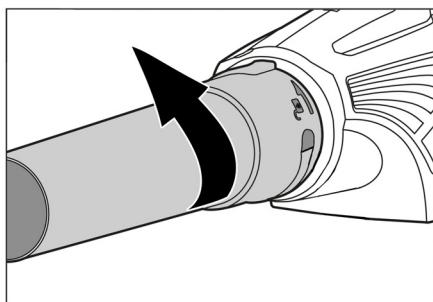
→ Turn the blower pipe in a counter-clockwise direction and remove it.
