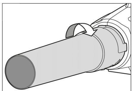
→ Turn the blower pipe in the clockwise direction to lock it (bayonet catch).
